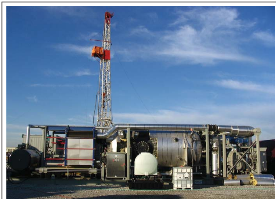
Aqua-Pure's processing systems use mechanical vapor recompression evaporation technology packaged in a self-contained, skid-mounted mobile unit that consists of a pretreatment module, an evaporator module and a compressor module.
